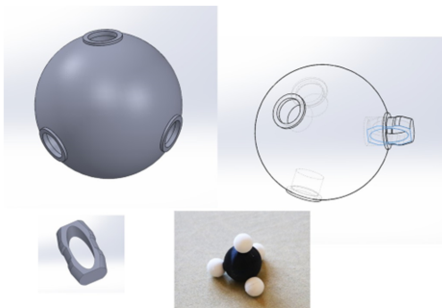
Figure 4 Model of the carbon atom, with the positions for the four single bonds (the model of methane CH 4 is also shown in which carbon is bonded to 4 hydrogen atoms) and the piece that we will use to join two atoms in a molecule.
